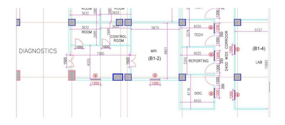
Indicative Lay Out Drawing for '3 Tesla-Magnetic Resonance Imaging (MRI) System'
